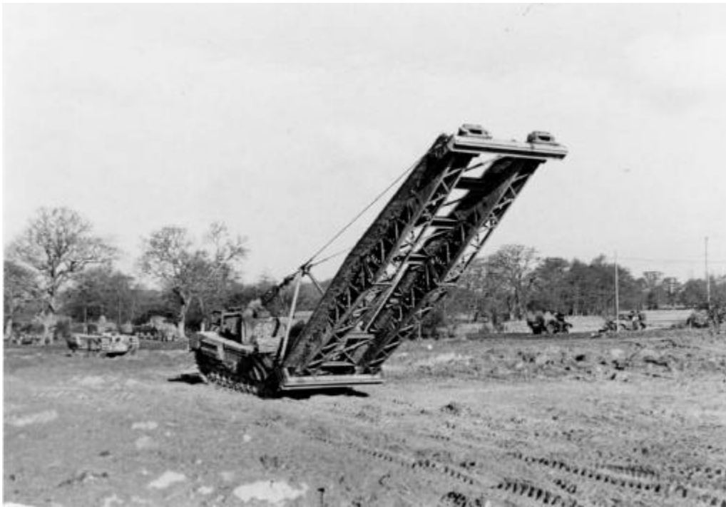
Fig. 3. AVRE deploying SBG bridge. Reprinted with permission of The Tank Museum, Bovington, Dorset, England.
